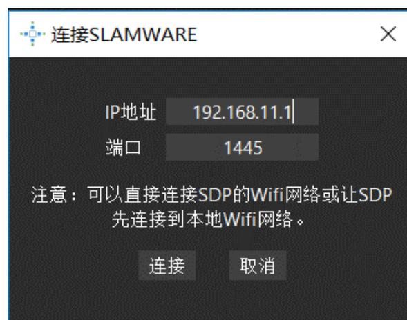
Figure 4-3 RoboStudio Robot Connection Dialog Box
